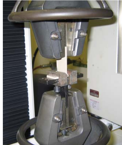
Figure 4 It shows how tensile test fixtures are designed and test was performed.
