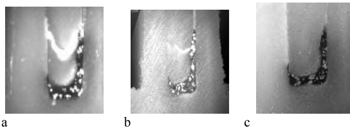
Figure 8. Tongue fractures a) nearer the tip of the tongue, b) nearer the root of the tongue, c) no tongue fracture evident
